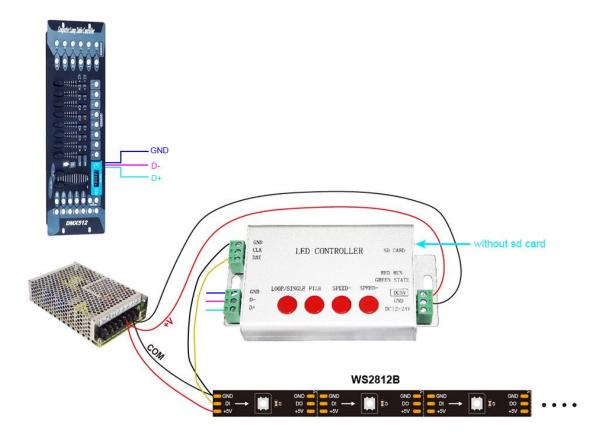
The chip type and clock of the control are obtained from the DAT file on the last inserted SD. The control output is from the address of the starting channel to 512 channels. The actual number of lamps connected can be less than that of the control output. When the total number of input channels is less than the initial channel address, the controller has no output.
