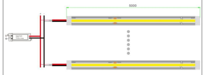
(PS: Strip positive connect to the driver positive, Strip negative connect to driver negative)
