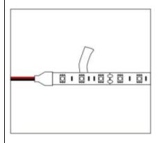
Do not release 3M paper by one time. No press on the leds
