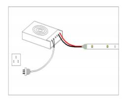
Connect the led strip wire to the driver output side (Positive to positive, negative to negative.)
