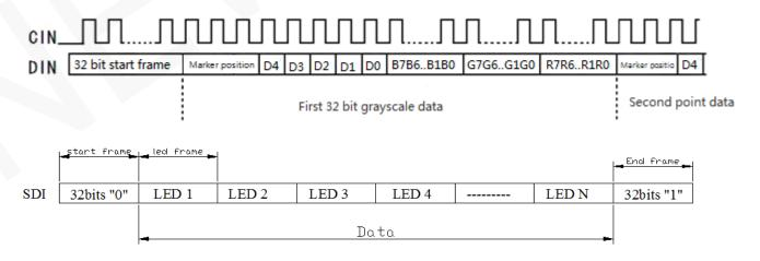
1. The first 32 bit "0" is the starting frame, and the CIN is on the rise time, and the timing DIN is preceded by CIN
