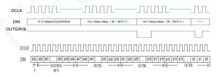
(A)first into at least 128bits "0" as the starting frame, and then moved into the data frame, the starting frame and the data frame are high first move in, DCLK rising edge sampling data:
